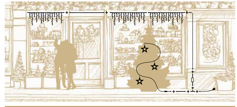
EXAMPLE OF MIXED 230V AND 24V WIRING
